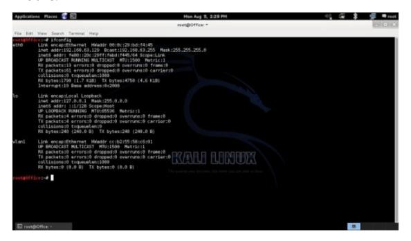
Most computers will give you three adapters: eth, lo, and wlan. For this task, you should focus on the "wlan" adapter. The image above shows that the name of the wireless adapter is "wlan1".
